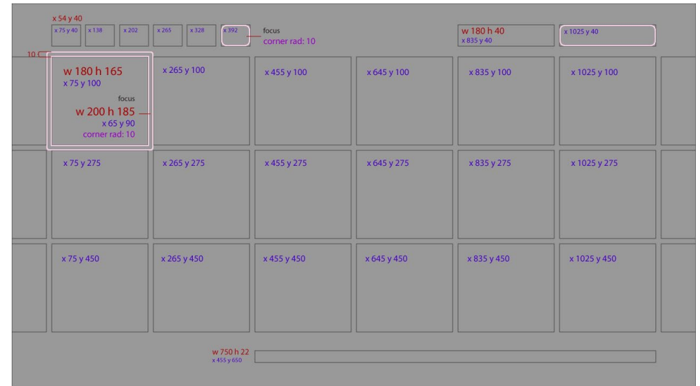
Measurements and positions of interactive elements (positions are the coordinates of the top left of each bounding box).
