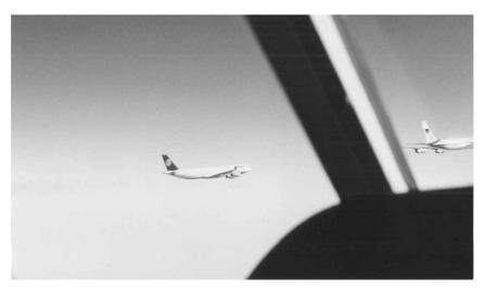
Fig. 2 Airbus A340 with contrails (left) and the Boeing B707 without contrails (right) taken from the Falcon research aircraft at about flight level 333 hft at 7:28 UTC, 15 Sept. 1999 (photographs: U. Schumann and R. Welser, DLR).
