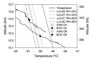
Fig. 4 Observed ambient temperature (thick curve) and threshold temperatures for contrail formation (thin curves) vs altitude, for various values of the overall efficiency  $\eta$  and ambient RH over liquid saturation: triangles pointing up and down are observed contrail formation conditions at ascent and descent, respectively.
